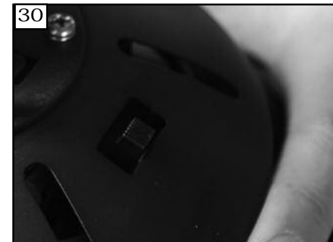
30 Reverse function for this fan is a switch on top housing of the fan body. Turn fan off and flip switch, this will reverse the direction of the blades.
